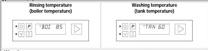
**Warning:** The tank and boiler temperatures shown on the display may be different from the actual temperatures by a few degrees, especially in transient phases (just after the FILL is completed, just after the end of the cycle, etc.) due to the inertia of the measurement probe.
